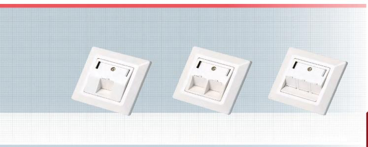
Data sockets consist of die-cast zinc frame and are suitable for installation in cable conduit, for flush mounting (FM), or surface mounting via separate frame. Installation as floor box also possible if 2 assembly tabs are broken off.
