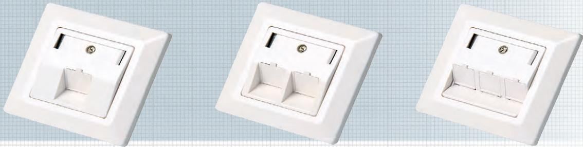
Data sockets consist of die-cast zinc frame and are suitable for installation in cable conduit, for flush mounting (FM), or surface mounting via separate frame. Installation as floor box also possible if 2 assembly tabs are broken off.
